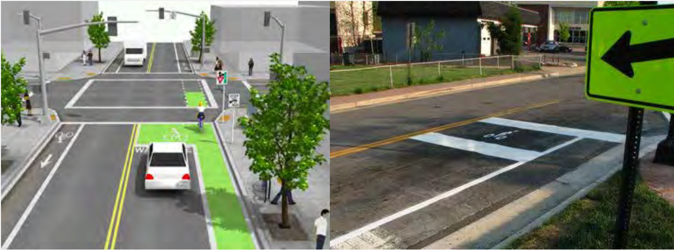
Figure 91: Bike Boxes. The model on the left (Image source: Richard Masoner ) shows the preferred design of bike boxes as specified in the NACTO Urban Bikeway Design Guide. The photo on the right (Image source: Blind Pilot ) shows a bike box installed on Commonwealth Avenue in Alexandria, Virginia.
